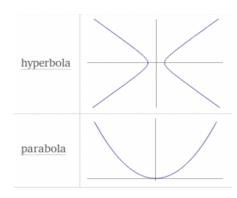
from there. The surface of this structure has a hyperbolic cross-section in one direction (if you look at the structure from above) and a parabolic cross-section in the other direction (if you look at the structure from the side), which gives it its name: hyperbolic paraboloid. It is shaped like a saddle or a Pringles chip.
