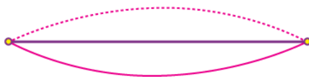
Figure 3: The fundamental wave formed when a string is plucked. This can also be formed by blowing into a flute, as the wave reflects off the walls of the instrument.
