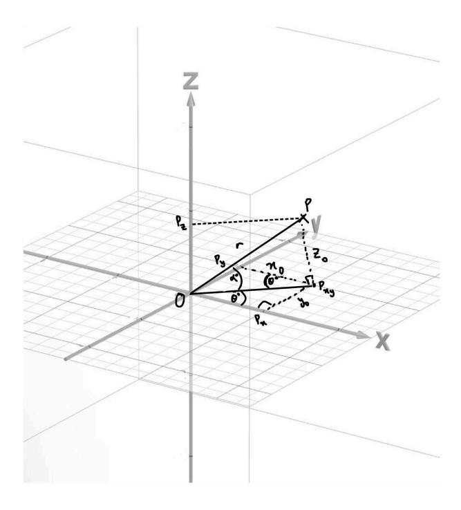
Multiple right angled triangles appear. The three relevant ones are triangle  $P_xOP_{xy}$ , triangle  $POP_{xy}$  and triangle  $P_yOP_{xy}$ . Expressions of  $x_0$ ,  $y_0$ , and  $z_0$  can be written in terms of r,  $\theta$  and  $\alpha$ . To do so for  $x_0$  and  $y_0$ , expression of  $OP_{xy}$  in terms of r,  $\theta$  and  $\alpha$  needs to first be determined. Focusing on triangle  $POP_{xy}$ ,
