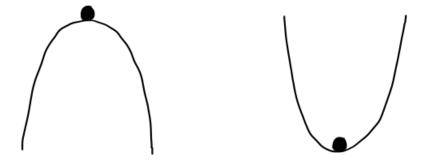
The diagram on the left represents instability. A small push of the ball from either side leads to it moving away drastically from the point it was previously on. The diagram on the right (stability) shows that the ball tends back towards the button of the curve.
