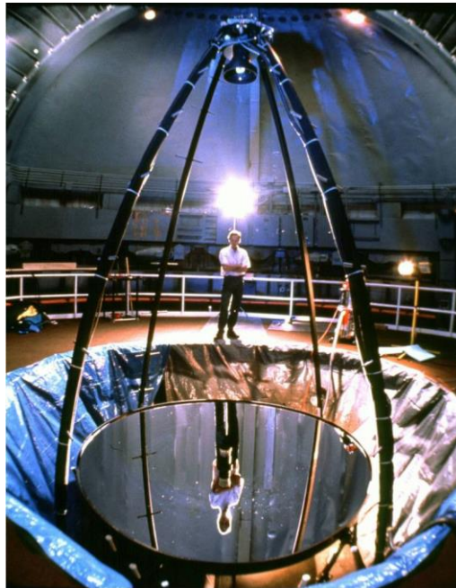
[Figure 16 – Liquid Mirror Telescope being used for a primary mirror with a rotating sensor]
