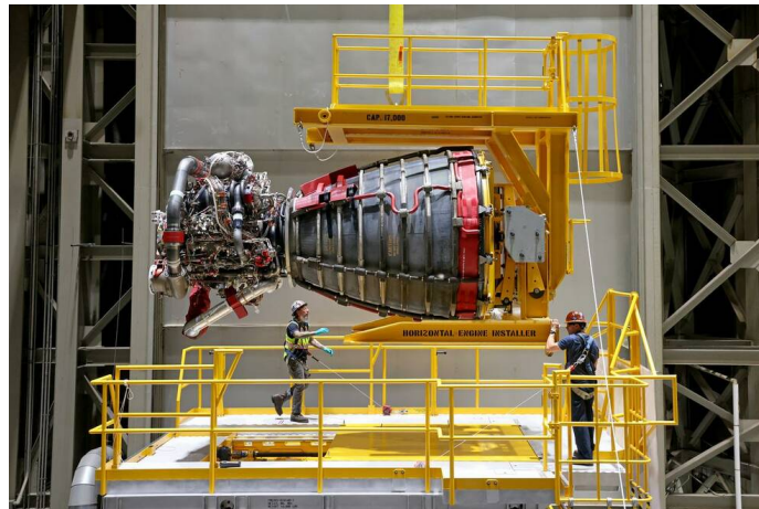
Figure 1: An RS-25 engine being attached to the Artemis II rocket. It has a de Laval shaped nozzle.
