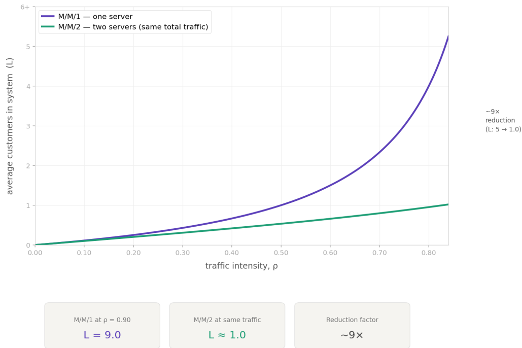
Figure 2: Average number of customers in the system ( L ) as traffic intensity \rho increases, for one server (M/M/1, purple) and two servers (M/M/2, green) handling identical total traffic.
