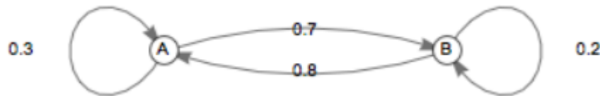
Figure 2: A simple two-state Markov chain. Even with random-looking moves, the system settles into stable proportions. (Note: Diagram values are illustrative)
